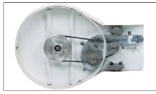
The design of the machine makes for easy access to the belt, drive pulley and vac. inlet. No high service labour costs. Longer life. Reduces likelihood of costly repairs.
